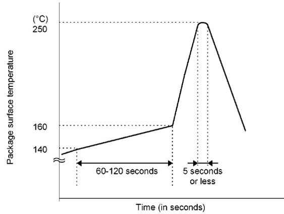
**Figure 3.5.5 Sample temperature profile for solder flow**
