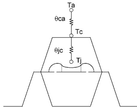
Figure 3.3.1 Thermal resistance of package
