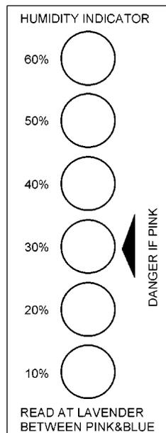
The indicator shown on the left can detect the approximate humidity level at a standard temperature of 25°C. When the ambient humidity is below 10%, all the humidity indicators will be blue.
