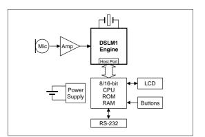
Figure 1. Modern IEC651 Type 0 / IEC804 Type 1 sound level meter application using the Xelentix's advanced DSLM1 DSP Engine
