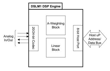
Figure 2. Functional block diagram of the Xelentix's advanced DSLM1 DSP Engine
