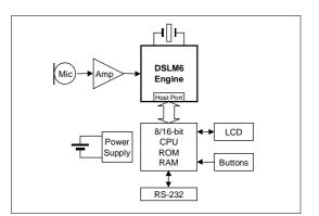
Figure 1. Modern IEC651 Type 0 / IEC804 Type 1 sound level meter application using the Xelentix's advanced DSLM6 DSP Engine
