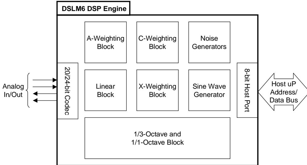
Figure 2. Functional block diagram of the Xelentix's advanced DSL6 DSP Engine
