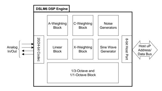
Figure 2. Functional block diagram of the Xelentix's advanced DSLM6 DSP Engine
