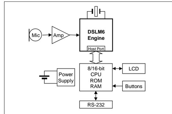
**Figure 1. Modern IEC651 Type 0 / IEC804 Type 1 sound level meter application using the Xelentix's advanced DSL6 DSP Engine**
