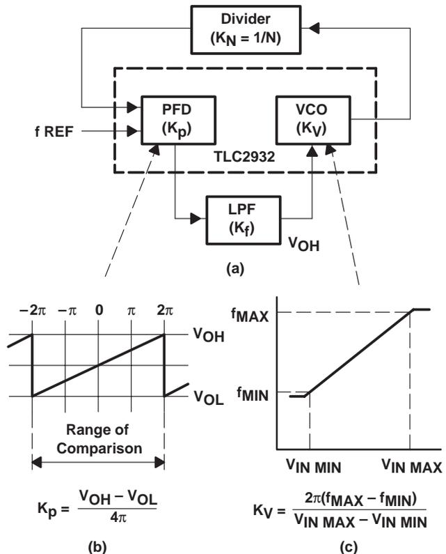
Figure 24. Example of a PLL Block Diagram
